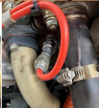
Photo 4: Spark plug in an awkward place.
