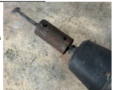
Photo 7: Spark plug cleaner tip fastens onto the vibrator. Colloquially at Hangar 64 this is an electric hamster back scratcher.
