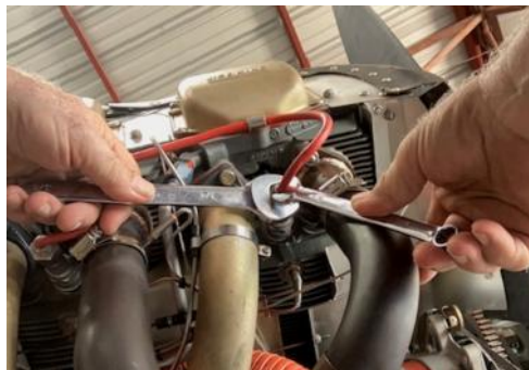
Photo 2: Wrenches on spark plug ignition lead.
