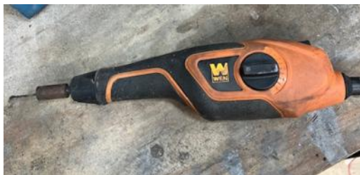
Photo 6: Vibrator – it is just a common engraving tool
