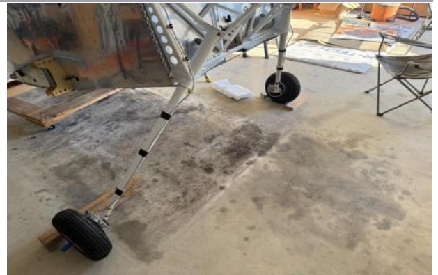
Wrapped the lines to the gear legs with friction tape.
