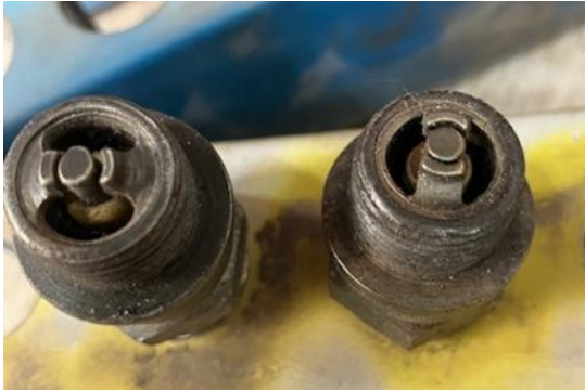
Photo 1: Massive electrode spark plugs, left is used/serviceable, right is new.
