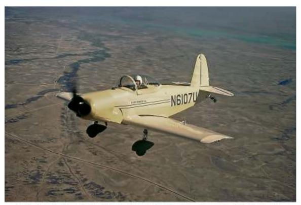
The Y2 undergoes further mods with a fully enclosed engine, spinner, and wheel pants that not only added to its attractive good looks, but increased speed and range as well. Photo taken over west Texas enroute to an Arizona aerobatic contest.
