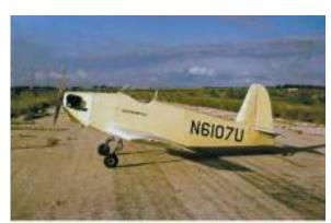
The Y2 as it appeared when making its first flight in September 1966 with open cockpit and exposed engine cylinders. Power was a Lycoming O-145 mounting a Moones Mite prop.
