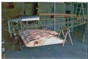
The single place Y2 under construction in late 1965. Note the simple fuselage structure and solid plywood ribs with routed sprace cap strips of the internally braced cantilever wing.
