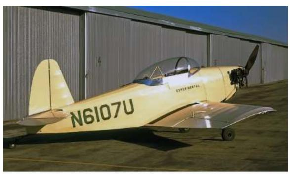
The Y7 flew most of its aerobatic contests in this configuration. Picture taken at Schlemeyer Field in Odessa in 1967. The canopy had just been installed, and the aircraft was now powered with a Lycoming O-190 G/D engine which provided improved aerobatic capability. A homemode prop was carved by Leon and proved very efficient.
